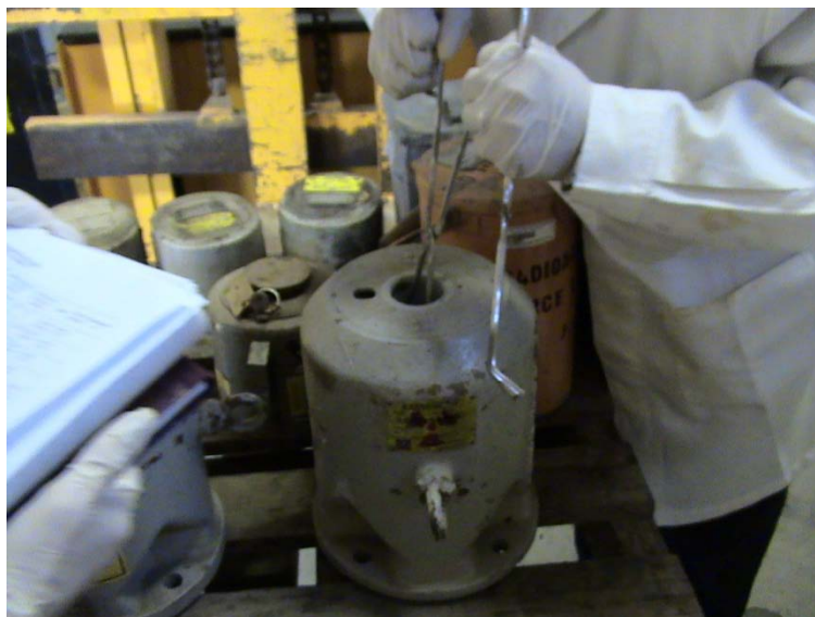
Figure 2: Removing Ra-226 brachytherapy source from storage shield in Chile.
