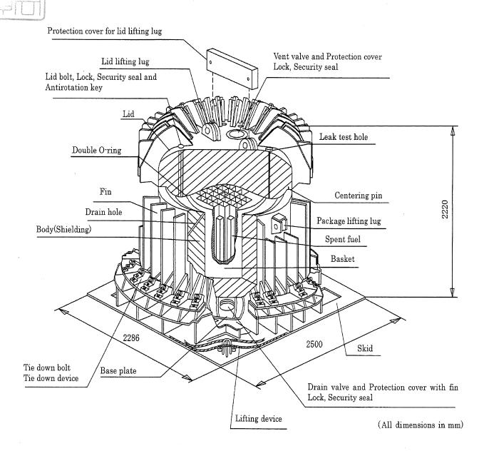
Figure-1 Illustration of JRC-80Y-20T Package
