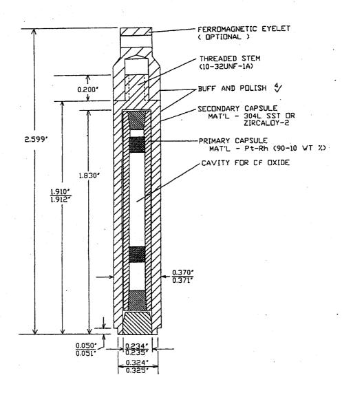
Figure 4. The primary and secondary capsule components (assembled) of the SR-Cf-3000 Series Source.
