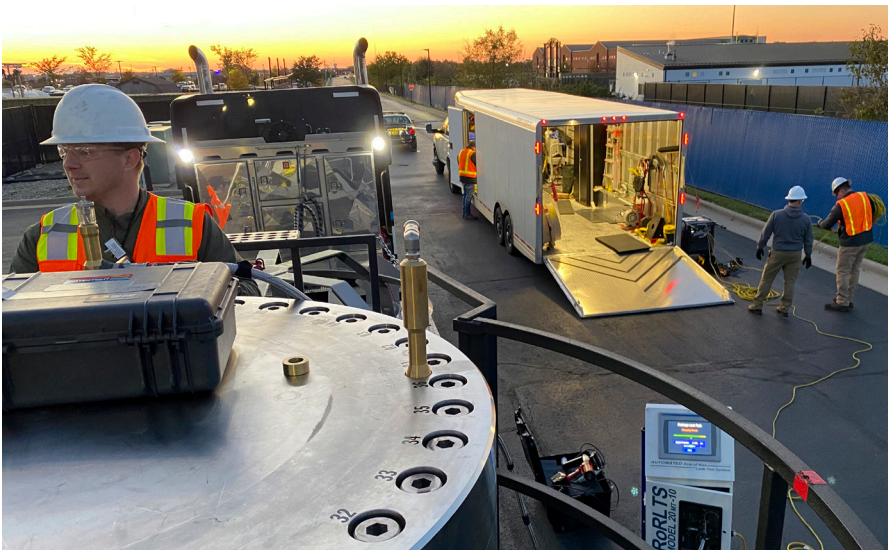
380B Type B Package undergoing pre-shipment leak test.
