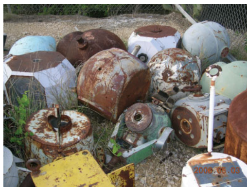
6 Incidents can occur if radioactive sources (or devices such as these teletherapy heads) are not properly dispositioned
