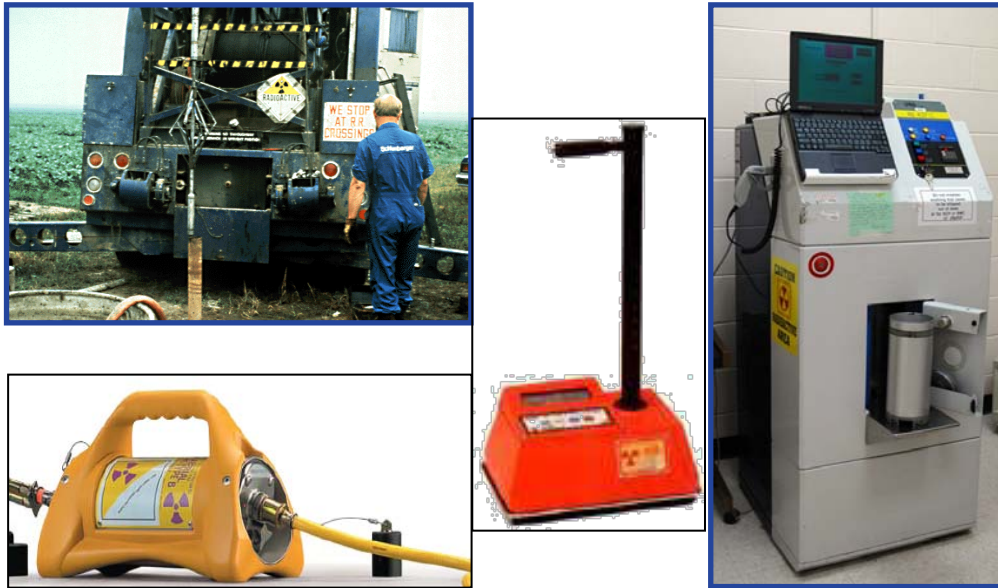
Figure 1: Beneficial Applications of Sealed Sources (Clockwise from top left). Well logging, Gauging (for moisture density and other types of measurements), Irradiation (blood), Radiography
