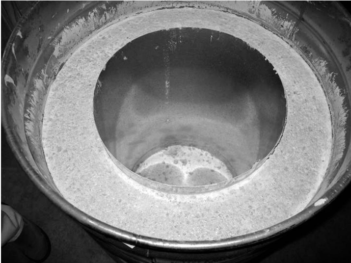
Figure 5: Interior Views of Two 55-Gallon Disposal Drums, One with a Large Opening for an Entire Disused Device and the Other with a Narrow Pipe Opening for Only Sources
