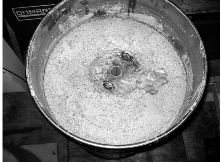
Figure 5: Interior Views of Two 55-Gallon Disposal Drums, One with a Large Opening for an Entire Disused Device and the Other with a Narrow Pipe Opening for Only Sources
