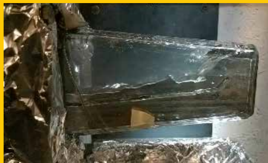
Flow visualization experiment of the Niowave molten lead-bismuth electron to neutron converter for Mo-99 production
