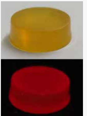
Initial QD-loaded composites show the material under room light (top), and a black light (bottom).
