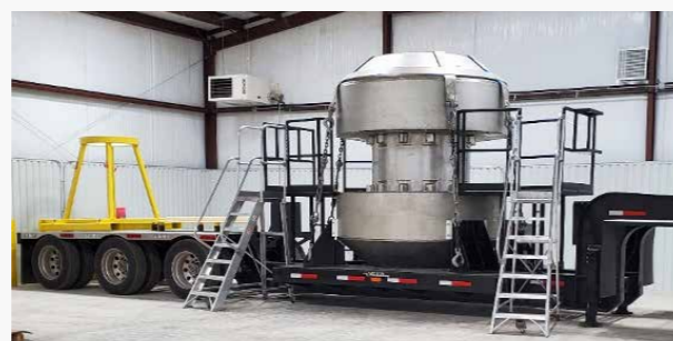
The 380-B is transported on a dedicated trailer outfitted with custom work platforms, lid stands, and impact limiter stands. The new container will be put into operation in 2021.
