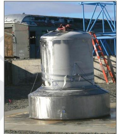
Photo of a half-scale test unit after a free drop test.
